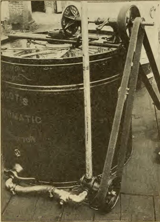
A closer view of the pump, showing the construction, method of belting, arrangement of pipe and hose connections and manner of tapping into honey-gate.
